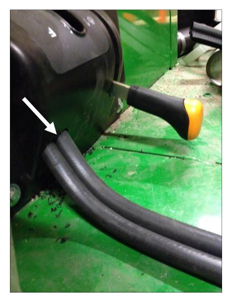
17. Pull the heater hose until the hoses are sitting nice and flat on the foot platform. Place the heater hose retainer cover onto the platform to locate the ideal location. The retainer will bend easily into place while locating onto the platform. Use the provided #8 screws to retain the hose ducting. Be CAREFUL when drilling holes through platform!
