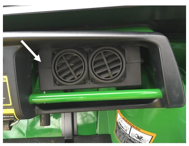
16. Route the heater hoses down from the glove box and rearward along the foot platform. Notch out the area in the center black plastic console for the heater hoses to run back into the engine bay as shown below.
