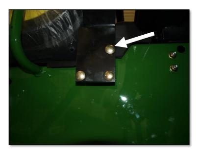
5. Using the top hole in the rear bracket as a guide, drill a 5/8" hole upwards through the fender plastic.
