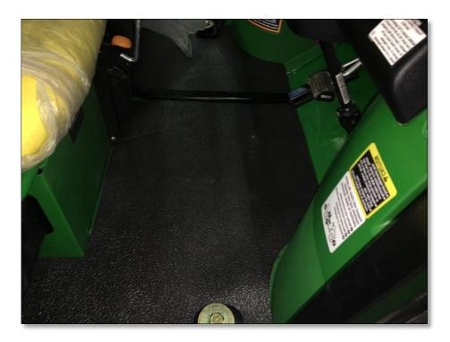
30. Use a black silicone seal and seal cab panels to the machine to minimize any locations of air and water entry into the cab.
