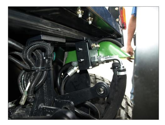
In order to use the back-hoe with cab, the rear window of the cab must be un-bolted and removed in order to allow the back-hoe seat to be installed.
