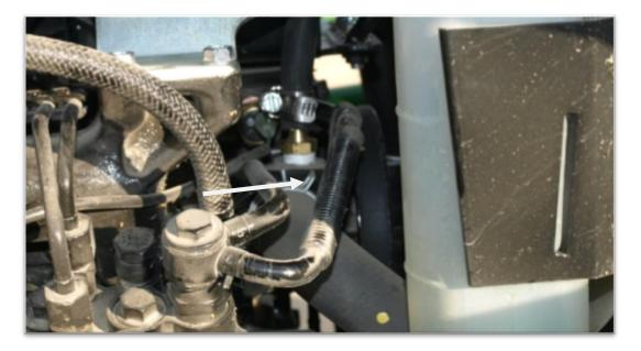
25. The suction fitting is located on the left side of the engine. Remove the muffler, then remove the plug indicated below. Use water sealant material around the threads of the fitting to prevent water leaks. Use the 16MM x 3/8" NPT straight fitting, brass o-ring, and screw it into the open port. Take the remaining 3/8NPT x 3/8" barb straight fitting and install into adapter. This is the suction fitting. Muffler MUST be removed to install.
