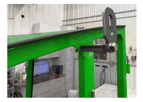
11. Attach a lift strap or chain to the lift brackets, and using a hoist or forklift, prepare to lift cab off of the shipping pallet. Un-bolt rear shipping bracket from cab, and lift cab. Position the cab over the tractor.
