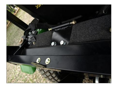
6. Re-install the control levers and end caps along with the tractor seat.
