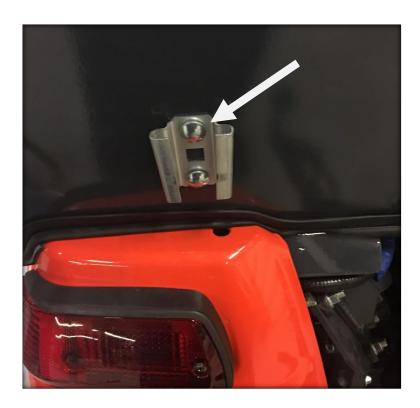
23. Take the SMV mount plate and apply bend to part that fits into sign mount. Adjust until such time that the SMV sign sits fairly straight when installed onto cab.
