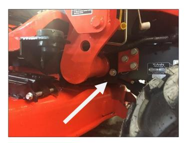
8. Take one of the rear brackets and slide it into the open socket where the 2-post ROPS was mounted on the left side. Use the factory hardware to fasten bracket to the tractor.
