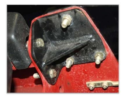
4. Take the right front bracket support and position it under the front right corner of the operator platform. Using the provided 3/8" x 1 ½" hex bolts and flange nuts, attach the bracket to the platform. See photo below of bracket installed.
