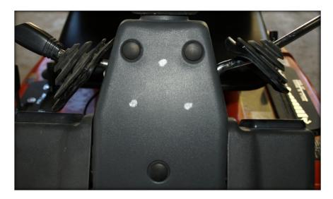
6. Position 4-way flasher mount bracket onto front of steering tower as shown and mark the three holes in the plastic as shown. Use care while drilling to ensure nothing else is damaged in the steering column. Drill 3/16" holes.
